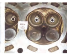
Combustion chamber after P.i. treatment.
