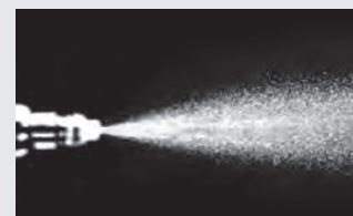
Injector spray pattern after P.i. treatment.
