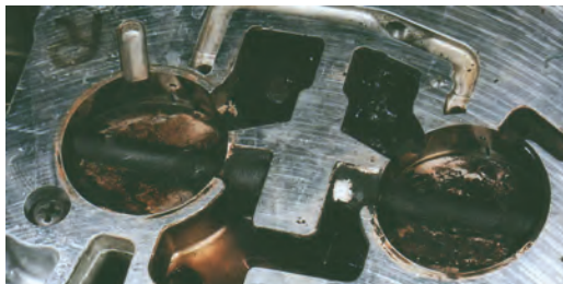
Picture J - Carburetor plates before P.i. treatment
