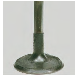
Picture E - Intake valve after P.i. treatment
