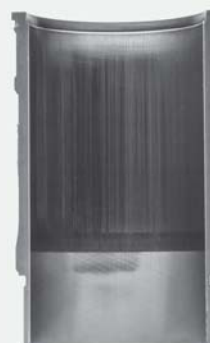
Severely Scuffed Liner
